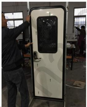
4. Use electric drill make holes to the in side door frame (four surface) (Each surface make two holes).
