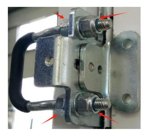
Step 9: Drill holes on the vehicle body based on the holes of the locking hook fixing plate, fix the locking hook fixing plate to the vehicle body with 4x16 self tapping screws, and tighten the locking hook fixing plate with a hex wrench.
