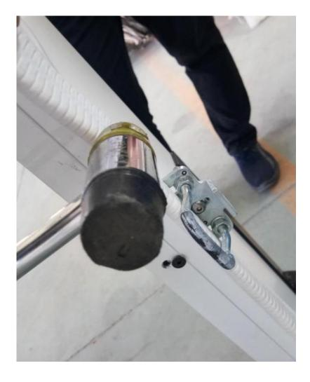
Step 7: Use scissors to cut off the interfering part at the locking hook position.
