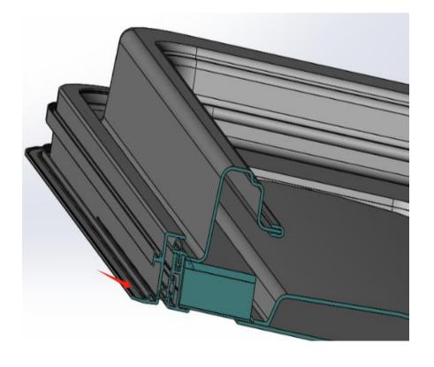
Step 3: Incline the door sideways into the hole of the vehicle body.
